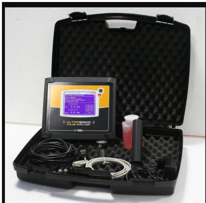
Figure 2: PULSONIC - Ultrasonic Pulse Analyzer Unit
