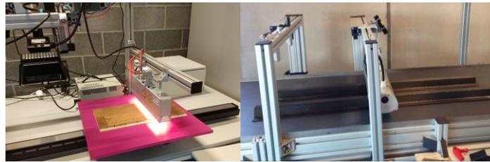
**Fig. 2:** Measurement set-up for dynamic line scan thermography on low speeds. The wooden samples translate beneath a heating source of 1 kW and are inspected using a thermal camera afterwards.
