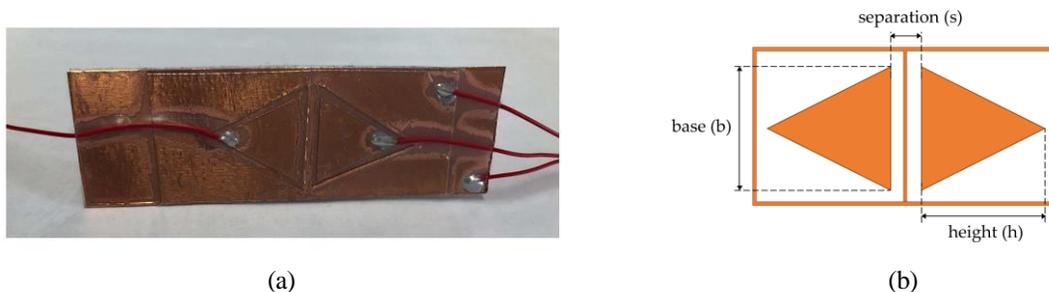
**Fig. 3** (a) Photograph of the pair of triangular electrodes and (b) Diagram of the capacitive sensor as viewed from the top surface.
