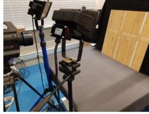
**Fig. 1:** Measurement set-up for pulse thermography inspections. The set-up consists of a cooled FLIR X6540sc camera, the wooden sample and a halogen tube lamp.
