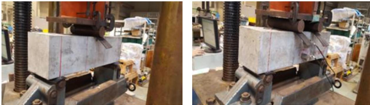
Fig 3.2 Concrete prism under three and four point loading and installed AE sensors on its surface
