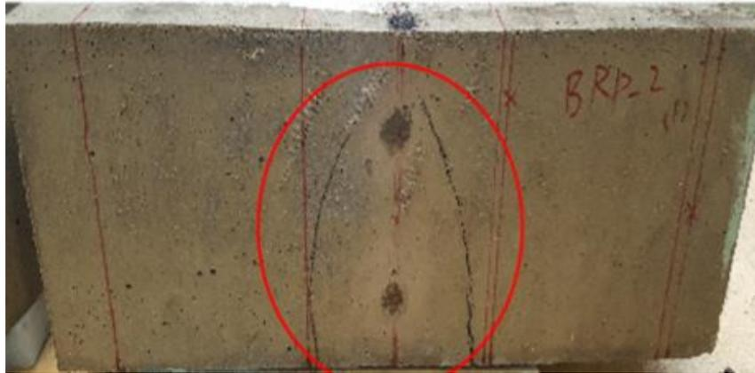
Fig. 4.6 Crack pattern in BRP-2 beam after peak application of peak load in three-point loading.
