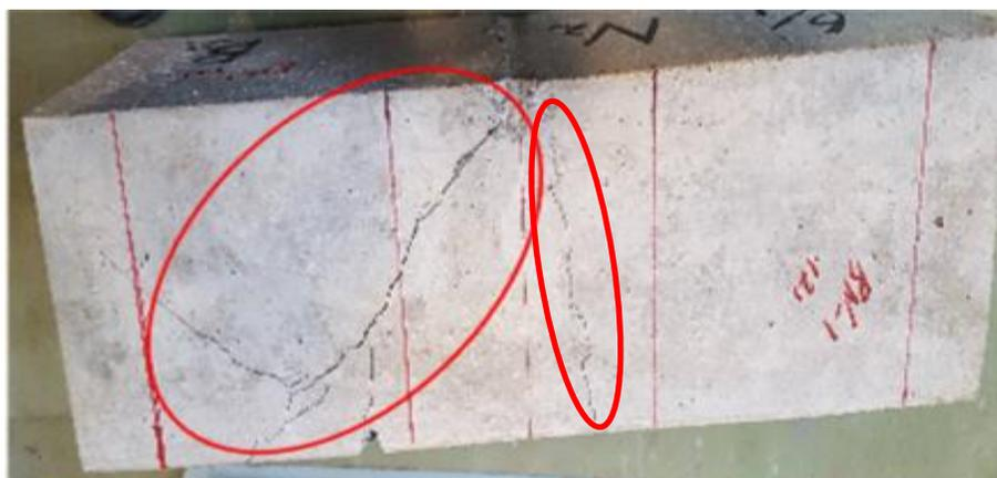
Fig. 4.5 Crack pattern in BN-1 beam after applying maximum cyclic three-point loading.
